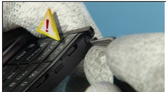
20. Repeat this procedure at the other side of the BOTTOM KEYMAT.
